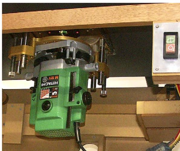
*Hitachi M12V mounted to a very substantial Woodpeckers Unilift. Note the 'no-voltage release' on/off switch at front RHS of table*
