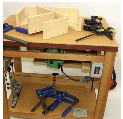
*Auxiliary 6mm MDF top locates with dowells at each corner to protect router and laminate top. Stretchers located some 50mm under top allow clamping from all four sides*
