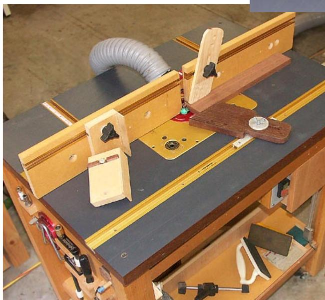
LE Aluminium fence with shop made T channelled MDF slides, feather boards and work stops. Note tool rack on LH side of table.
