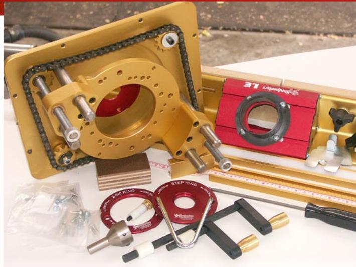
*The Woodpecker's Unilift lift and LE Router table fence as supplied. The router's base plate is removed so that it mounts directly to Unilift. Note robust construction and bearings. Scaletrack, composite base panel and collet extension are extra, but you can live without them. I found the XTreme collet extension caused bad vibration and was not really needed.*
