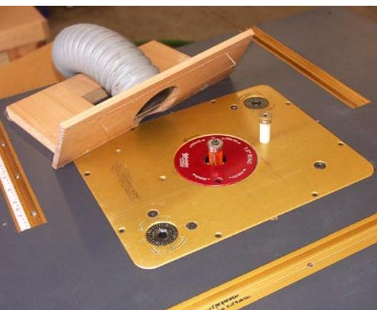
Similar convenience and safety features apply when insert rings are used in conjunction with the supplied starter pin for freehand or bearing guided pattern following work. The shop made Super Scooper dust collector comes into its own for these tasks.
