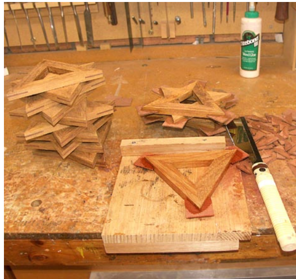
Trimming splines to about 3mm from trivet sides
