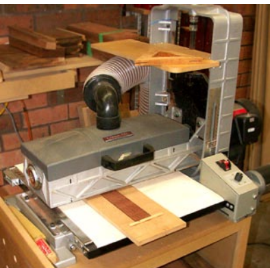
Drum sanding stock to final thickness for mitre splines. Note: MDF sled which allows accurate tolerances at this fine thickness and the test trivet sitting on the WIP rest for constant checks on fit - see text.
