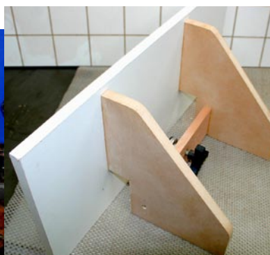
L. Re-sawing with an auxiliary fence. R. Auxiliary fence made from 16mm melamine faced chipboard - slips snugly over the saw's supplied fence.
