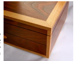
Walnut with Silky Oak mitred lipping and corner posts to conceal veneer edges - Reg Orr.
