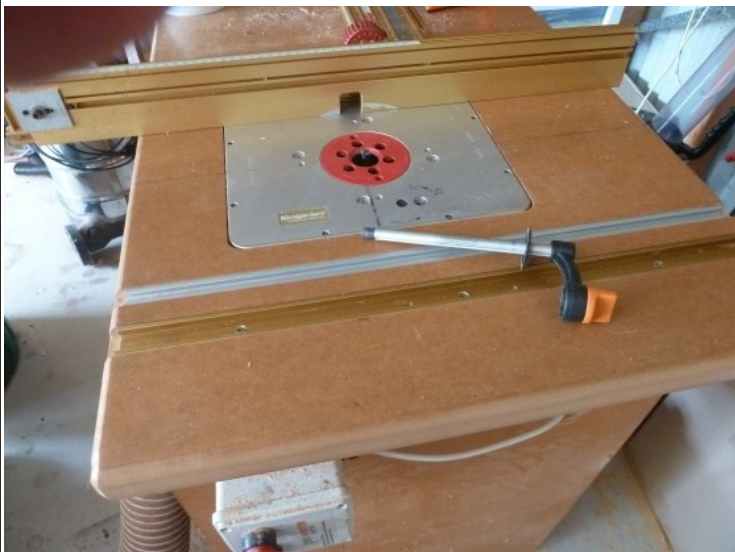
Note the holes drilled in the insert
