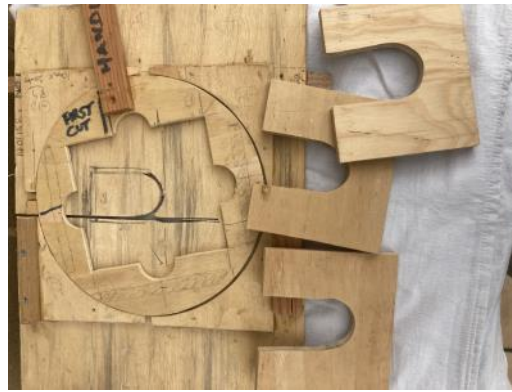
Phil Leach's birdbox-window-cutting jig on the job
