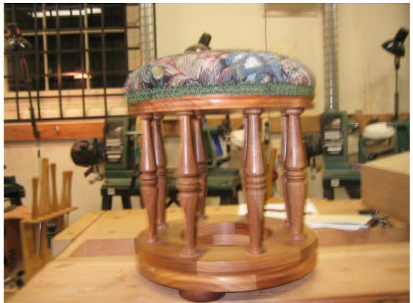
Above is pictured the Foot stool which we are making in Manningham woodturners as mentioned in the article at left. The base consists of a ring which in this case is laminated, with a solid top.
