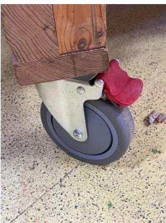
NOTE: the braking system on the new castors is a little different to the old ones and works with TWO levers – the top one for brake OFF and the bottom one for brake ON.
