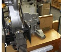
3. Hinged LHS table top fence, up. 4. Fence flipped back to allow saw to tilt left.
