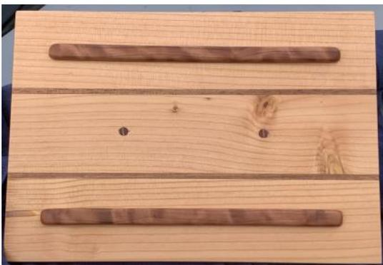
I attached the handle to the mounts/tomb stone looking things with some Red gum dowels I turned on the lathe of which I also used dowels to connect the tombstones to the lid and then put a contrasting wedge into them all.
