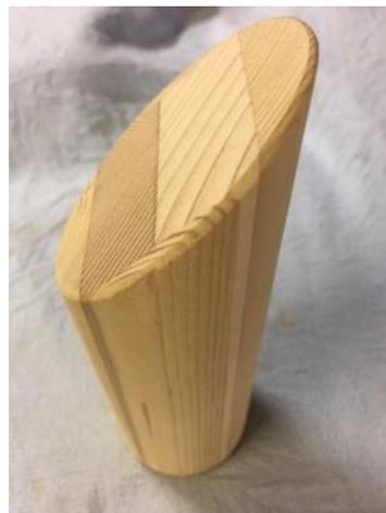
I let the glue set for 24 hours, then it was time to put the piece in the lathe. I used calipers to monitor the diameter to arrive at the 60 mm finished diameter.
