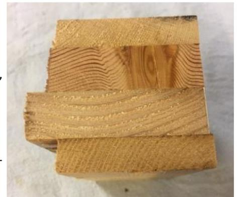
This photo shows the "square" shape of the 6 segments, about 69 mm wide (52 mm plus 2 x 8.5 mm) and 62 mm "high" (2 x 19 mm plus 2 x 13 mm).
