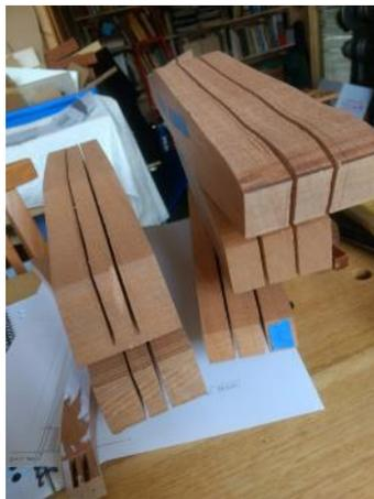
Then I sawed the rest of the way through using a Japanese pull saw, and planed each piece to a scribed thickness.
