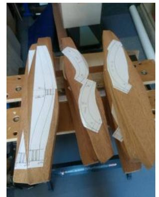
I've attached a cutting pattern to each piece, for each individual component. Now I just have to make lots of 4mm wide tenons and mortises so that I get joints like this test I made.
