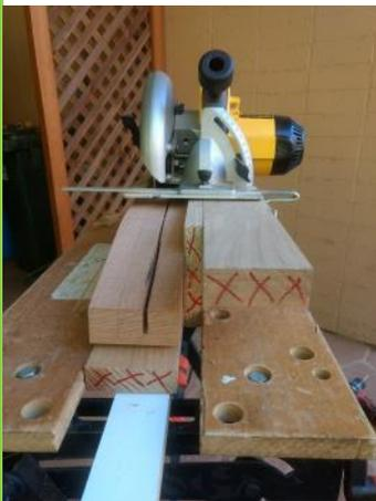
I made a safe, secure jig to rip the slabs with my circular saw, about 2/3 through. Jig is marked with red X.
