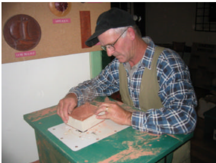
Charlie Chamberlain during the box making course. He's routing out a groove to fit the bottom and top onto
