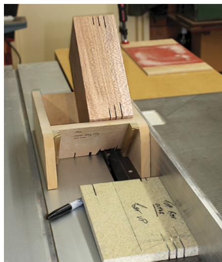
Hold the jig and box tightly to the fence throughout the cuts for consistent kerfs and well fitting keys. Remove the set-up block before you start.
