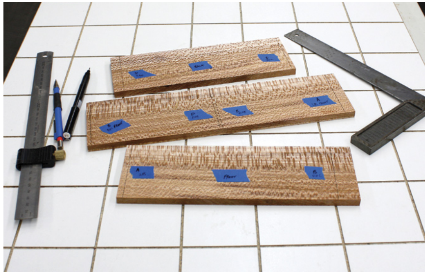
Pic 2: Yet another piece of blue masking tape (with a cross), indicates which face and side not to rabbet when routing the base rebates. You can rabbet prior to cross cutting when working with one long piece, as the rebates can run right through the ends.
