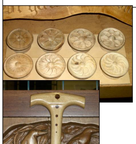
The knobs displayed on this page demonstrates step by step how they were made. Starting from the left from a turned plain knob to the completed item on the right.
