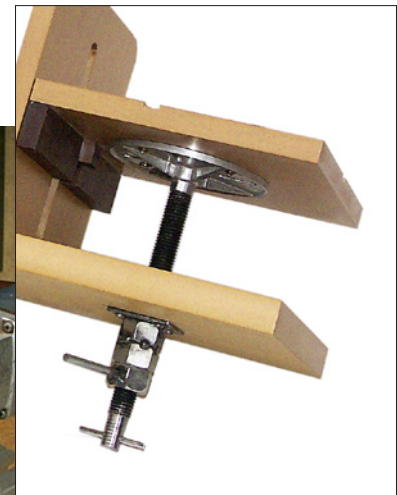
Pic #8 Feed table height adjustment mechanism with levered locking nut.
