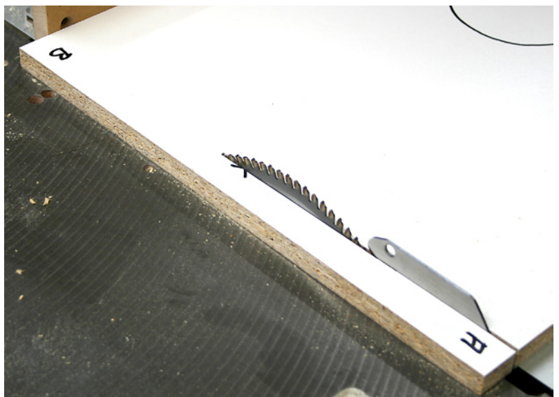
Pic 5 A 20mm test strip is cut off edge X. Before cutting, mark it A on the leading face and B on the trailing face.
