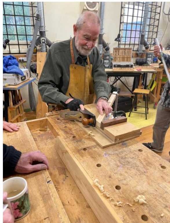
John Paine (Thursday PM) with a couple of his planing jigs—wedged board holder, and shooting board.
